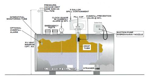
Aboveground Bulk Tank with Remote Pump(s)
