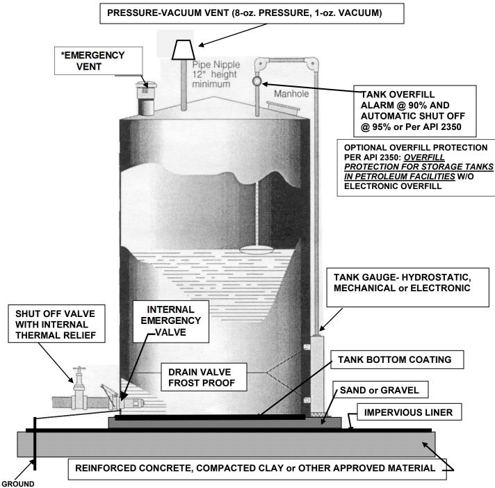
\*Emergency relief venting consists of a manufactured emergency vent to relieve at approximately 2.5 psig pressure, or refer to liftable manhole covers, large diameter vents or weak roof to shell welds if either of these alternatives is used. NC Fire Prevention Code (IFC) Sections 2306.6.2.6 and 5704.2.9.6.8 requires a fixed 5-gallon spill container to be attached to the fill pipe on top of tanks or portable spill containment will be allowed for tanks with remote fill connections.
